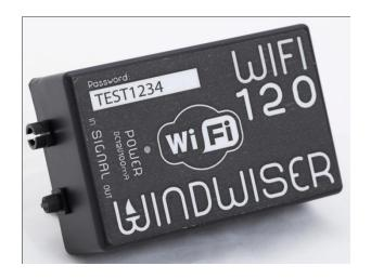
The Windwiser 120 W Wifi module is a simple unit to integrate into the CAN communication system of the device. It converts the measured data into a standard Wifi signal and transmits it as a NMEA0183 message. The signal can be received by a mobile device or tablet and displayed using Android or IoS applications. The data from your boat is saved by the apps so it can be viewed later. The apps can even display the polar diagram of your boat.
