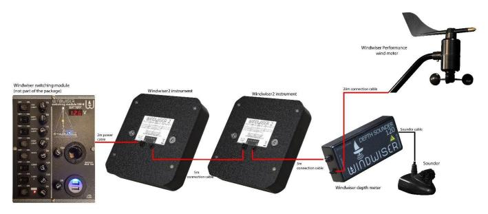
At the end of the installation, when you switch on for the first time, check that the wind gauge reads 0° in a headwind. If the AWA is not 0° in a headwind, the calibration can be done as described in the "Setup and Calibration" menu.
