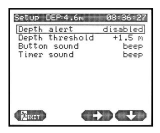
**Depth alert**: Sets the depth alarm mode. If the depth gauge measures a depth less than the depth set in the "Depth threshold" menu item, there are three ways the device can react: in "disabled" mode, no depth alarm; in "beep" mode, when a depth alarm is triggered, it will continuously emit a short, intermittent beep while the depth display in the upper information bar flashes; in "silent" mode, no beep, only the depth display in the upper information bar flashes.
